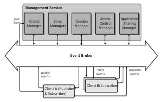
Figure 2. The architecture of NVEs on VRWork
